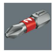
BiTorsion bits are absolutely premium products. They have a softer BiTorsion zone which reduces the hardness of the shaft by about 20 % in comparison to the drive tip. This means that the peak loads that cause bit breakage and premature wear are absorbed in this zone - something which enhances the service life of the
